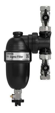
A high-performance, magnetic in-line system filter, the TF1 Sigma Filter is ideal for restricted spaces as it is capable of multiple orientations. This simple to install, composite plastic filter fits onto vertical and horizontal pipework, and works by allowing hydrocyclonic action to deliver contaminants to the unit's powerful magnet assembly for safe removal.
